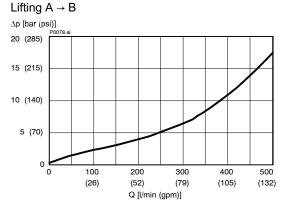
$\Delta p = f(Q)$  Pressure drop - Flow rate characteristic Lowering B  $\rightarrow$  A, valve fully opened
